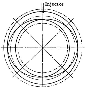
We note that the number of electrons missing the injector increases as the square of the emission current of the injector. Taking into account the influence of the Coulomb repulsion, the number of captured electrons will be proportional to the fourth power of the emission current as the result of the decrease of the energy of the radial oscillations. This agrees with the experimental results.
