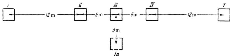
FIG. 1a. Arrangement of the groups of hodoscope counters.
