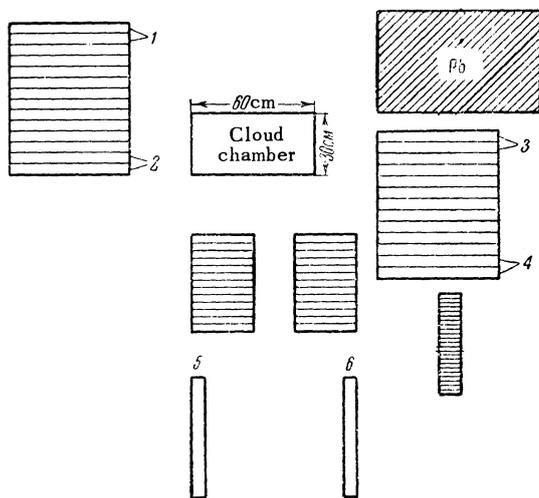
FIG. 1b. Arrangement of the hodoscope counters and cloud chamber in group III.
