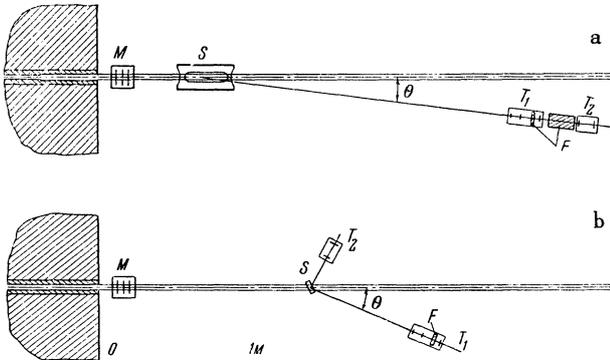
FIG. 1. Experimental setup. M—Monitor, S—Scatterer, T<sub>1</sub>, T<sub>2</sub>—telescopes, F—copper absorber.
