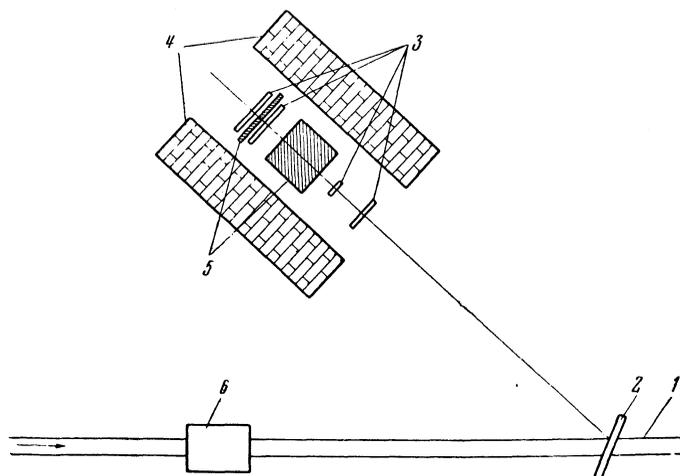
FIG. 1. Experimental setup. 1—proton beam; 2—target; 3—scintillation counters; 4—lead shield; 5—copper or aluminum filters; 6—monitor.
