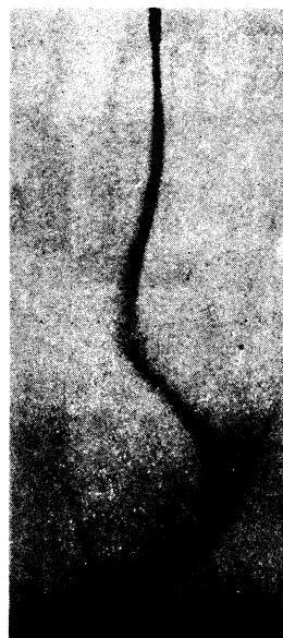
FIG. 2. Breaks in the jet of the electrolyte in an electric field of moderate intensity; electrodes on the right and on the left. Scale 2:1.
