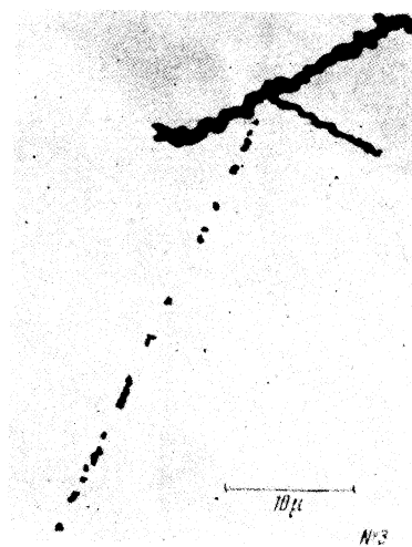
FIG. 3. Fission of a uranium nucleus by a fast neutron accompanied by the emission of a 16 mev proton and an \alpha particle of energy greater than 8 mev.
